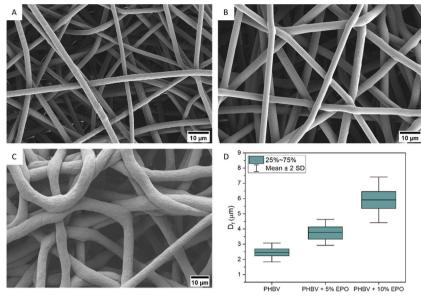
Fig. 1 (A) SEM micrographs of the PHBV fibers and (B) blend PHBV fibers with 5% EPO and (C) 10% EPO. (D) Box chart with the mean diameter values (D<sub>f</sub>) of the fibers and the interquartile interval in the PHBV electrospun scaffold and blends with 5% and 10% EPO.
