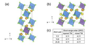
Fig. 6  $Na_{2.25}Y_{0.25}Zr_{0.75}Cl_6$  structural models with different Y–Zr orderings. Color legend: Y is purple, Zr is light blue, Cl is light green, while Na in an octahedral or prismatic environment is yellow and orange, respectively. The two types of Y-Zr orderings are referred to as (a) layered-TM and (b) mixed-TM structures. (c) Short-range order (SRO) parameters that describe Y-Y, Y-Zr and Zr-Zr correlations. These SRO parameters are defined in the Methods section.
