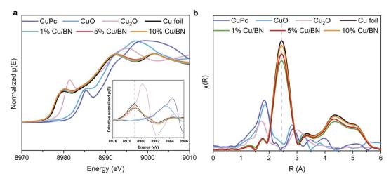
Fig. 3 XAS characterisation of Cu/BN samples with varying Cu contents and reference samples. (a) Normalised Cu K-edge XANES spectra; inset: derivative Cu K-edge spectra; (b) phase corrected  $k^2$ -weighted Fourier transformed EXAFS spectra, using k-range 3-11 Å<sup>-1</sup>.
