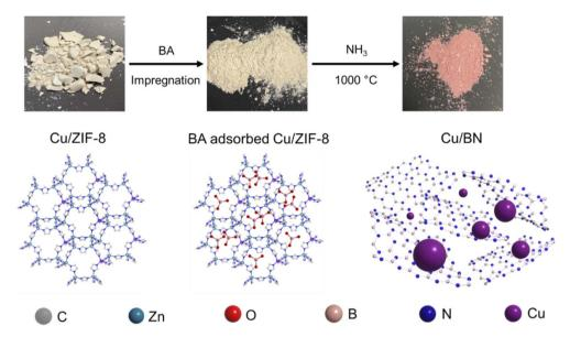
Scheme 1 Schematic representation of Cu/BN synthesis
