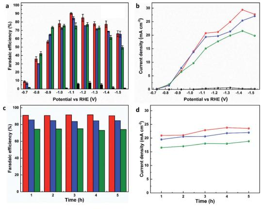
Fig. 3 Catalytic performance of MFM-220-p/CP (red lines or column), MFM-221-p/CP (blue lines or column), MFM-222-p/CP (green lines or column), and CP (black lines or column) electrodes for  $CO_2RR$  in 0.1 M KHCO<sub>3</sub>. Plots of (a) FE<sub>formate</sub> vs. potential, (b) current density for formate production vs. potential, (c) FE<sub>formate</sub> vs. time, and (d) current density of formate vs. time for reduction of  $CO_2$  at -1.1 V vs. RHE.
