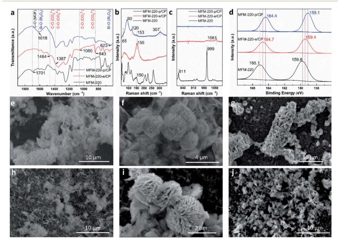
Fig. 2 Characterisation of the transformation and evolution of Bi-MOFs to  $Bi_2O_2CO_3$  nanosheets and  $\alpha$ - $Bi_2O_3$ . (a) FT-IR spectra; (b and c) Raman spectra; (d) XPS spectra; SEM images of (e) MFM-220-e/CP, (f) MFM-221-e/CP, (g) MFM-222-e/CP, (h) MFM-220-p/CP, (i) MFM-221-p/CP, and (j) MFM-222-p/CP.
