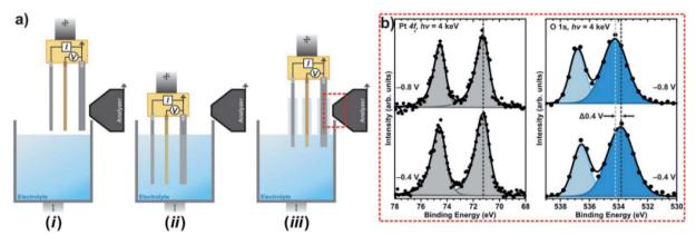
Fig. 31 (a) Illustration of the electrolyte beaker and electrode housing used for the dip-and-pull method. (b) Pt 4f and O 1s spectra recorded at two different voltages. A shift in energy is seen for the O 1s peak stemming from the electrolyte, while the Pt signal (stemming from the working electrode) remains fixed. Reproduced under CC-BY licence from ref. 214.
