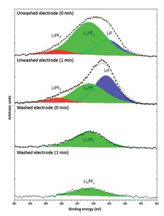
Fig. 6 F 1s XPS spectra (Al Kα, 1487 eV) from washed (dimethyl carbonate (DMC), 2 min, dried in argon) and unwashed graphite anode from full cells with LiCoO2 cathode and electrolyte of 1 M LiPF6 in ethylene carbonate (EC)/ethyl methyl carbonate (EMC), 3:7 w/w. The minutes in the figure refer to the duration of Ar<sup>+</sup> sputtering before XPS measurement. Reproduced under CC-BY licence from ref. 66.
