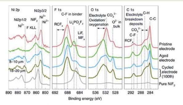
Fig. 10 XPS spectra (Ni 2p, F 1s, O 1s, C 1s) of LiNi<sub>0.7</sub>Mn<sub>0.15</sub>Co<sub>0.15</sub>O<sub>2</sub> electrodes (pristine, aged, and cycled electrodes with 8–10 and 18–20 µm particle sizes) and pure NiF<sub>2</sub>. Reproduced under CC-BY licence from ref. 107.
