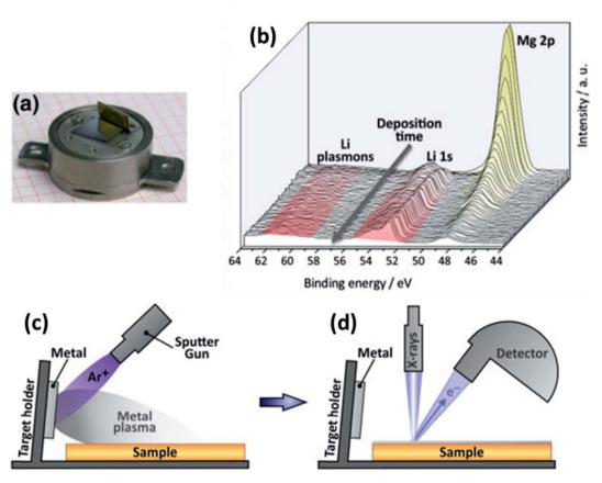
Fig. 25 An experimental set-up for *in situ* XPS. (a) Modified XPS sample holder with electrode active material target. (b) Calibration XPS measurement of Li sputtering onto MgO substrate. (c) Illustration of the *in situ* sputtering using an ion gun. (d) Illustration of the XPS analysis after *in situ* sputtering. Reprinted from ref. 175, with permission from Elsevier.
