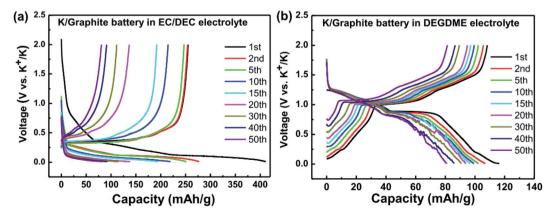
Fig. 15 Galvanostatic voltage profiles for K/graphite cells using (a) carbonate, and (b) ether electrolytes. Reprinted from, 148 with permission from Elsevier.
