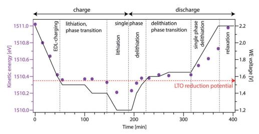
Fig. 34 Kinetic energy of the electrolyte peaks as a function of time (purple dots) and WE voltage as a function of time (black line). The kinetic energy shifts of the electrolyte are different depending on the type of reactions occurring at the WE/electrolyte interface. Reproduced under CC-BY licence from ref. 228.
