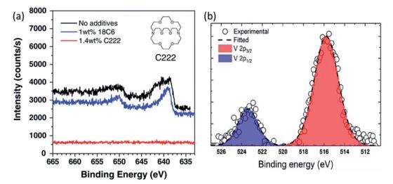
Fig. 12 (a) Mn 2p spectra of graphite electrodes after 5 cycles with LiMn<sub>2</sub>O<sub>4</sub> cathodes in 1 M LiClO<sub>4</sub>/EC + DEC with and without the 18C6 or C222 cyclic ether additives. Reproduced from ref. 119 with permission from the Royal Society of Chemistry. (b) V 2p core level of the vanadium deposited on the anode. Reprinted with permission from ref. 122. Copyright 2019 American Chemical Society.
