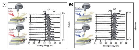
Fig. 27 In situ XPS set-up using a "virtual electrode" and the resulting spectra in (a) charge and (b) discharge. Reprinted from ref. 196, under a CC-BY license.
