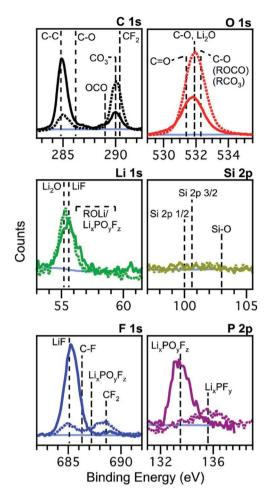
Fig. 4 XPS spectra of silicon (001) wafer electrodes after preparation by chronoamperometry at 0.01 V vs. Li<sup>+</sup>/Li for 300 s in an electrolyte of 1 M LiPF<sub>6</sub> in ethylene carbonate (EC) and diethyl carbonate (DEC), 1:1 w/w. Solid lines: measured without exposure; dashed lines: measured after exposure to the atmosphere for 10 minutes. Reprinted with permission from ref. 56. Copyright 2012 American Chemical Society.
