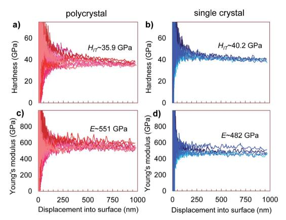
Fig. 5 The nanoindentation hardness,  $H_{\rm IT}$  (a and b), and Young's modulus, E (c and d) of polycrystals (a and c) and single crystals (b and d) of WB<sub>4</sub> at 295 K. Each plot combines several tests and shows average values.
