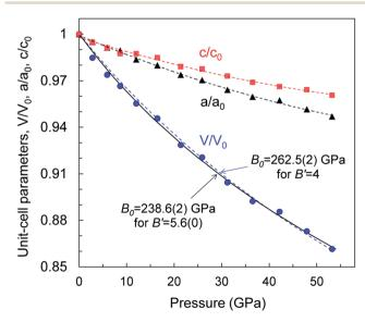
Fig. 4 Pressure dependencies of relative variations in the unit-cell volume and lattice parameters of a  $WB_4$  single crystal at 295 K. Error bars are smaller than symbols' size.
