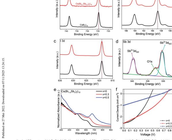
Fig. 2 XPS spectra of (a) Cs 3d, (b) Bi 4f, and (c) I 3d of CBI and CBSI-3 films, and (d) Sb 3d of CBSI-3 film, (e) UV-vis spectra of CBI, CBSI-3, and CBSI-5 films on the ITO/PEDOT substrate. (f) J-V curves of CBI, CBSI-3, and CBSI-5 devices with an inverted device architecture (ITO/PEDOT/ CSBI/PCBM/bathocuproine (BCP)/Ag) measured under illumination (AM 1.5G, 100 mW cm $^{-2}$ ). All films illustrated here are synthesized from DMF/ DMSO mixed solvent with volume ratio of 9 · 1
