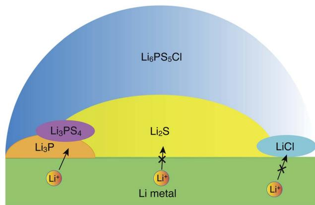
Fig. 5 Schematic illustration of a possible structure of the interface between Li metal and argyrodite- $\text{Li}_6\text{PS}_5\text{Cl}$ , as inferred from the interfacial energetics and Li-ion transport simulations.
