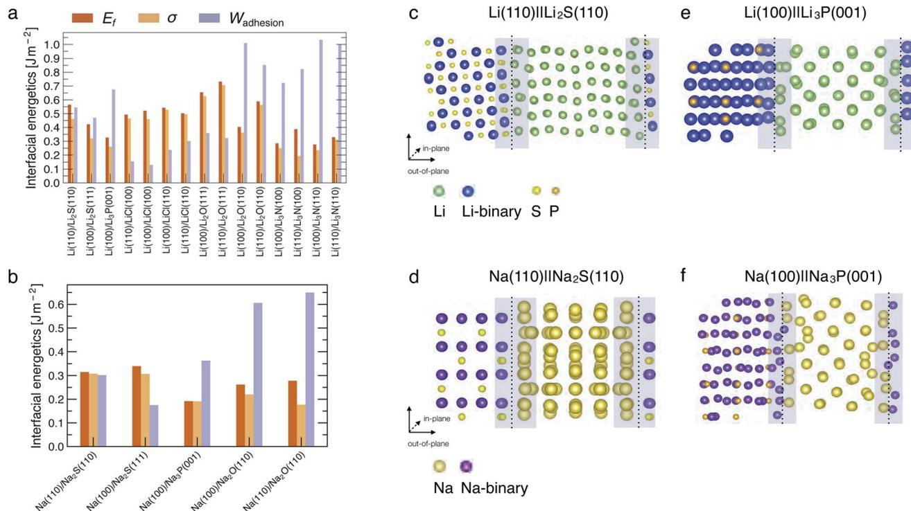
Fig. 2 Computed interfacial quantities (in  $\text{J m}^{-2}$ ) for (a) Li-based interfaces and (b) Na-based interfaces. Atomic structures of representative interfaces, namely (c) Li(110)||Li<sub>2</sub>S(110), (d) Na(110)||Na<sub>2</sub>S(110) (e) Li(100)||Li<sub>3</sub>P(001) and (f) Na(100)||Na<sub>3</sub>P(001). The interface regions are indicated by the shaded areas. The non-periodic direction of the interface is indicated by the "out-of-plane" vectors.
