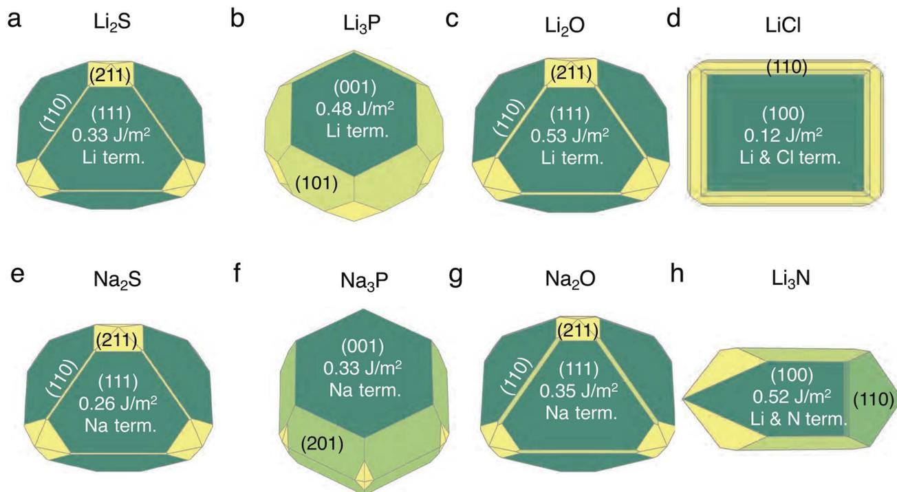
Fig. 1 Computed Wulff shapes of binary compounds Li<sub>2</sub>S (panel a), Li<sub>3</sub>P (b), Li<sub>2</sub>O (c), LiCl (d), Na<sub>2</sub>S (e), Na<sub>3</sub>P (f), Na<sub>2</sub>O (g), and Li<sub>3</sub>N (h), with their corresponding surface energies (in J m<sup>-2</sup>). The chemical nature of the surface terminations (term.) are also indicated. Wulff polygons are constructed using stoichiometric, non-polar, and symmetric surfaces (including an inversion symmetry).
