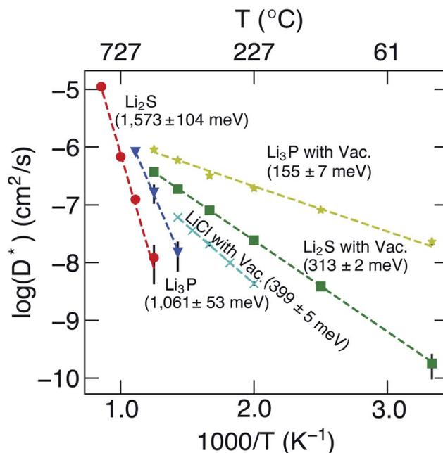
Fig. 3 Arrhenius plots of  $\text{Li}^+$   $D^*$  (in  $\text{cm}^2 \text{ s}^{-1}$ ) of bulk binary compounds from MTP-MD simulations. The activation energies, calculated from eqn (7), and the related error bars are provided as text annotations. Vac. stands for structures with a Li vacancy.
