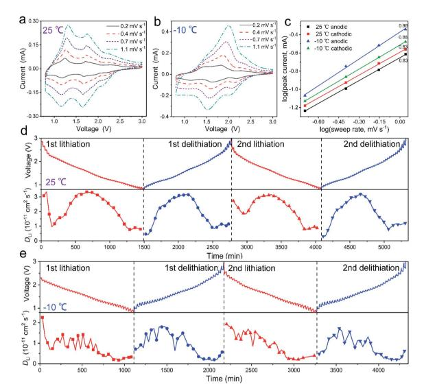
Fig. 5 Electrochemical kinetics of  $Mo_4Nb_{26}O_{77}$  submicron-sized particles. CV profiles of the  $Mo_4Nb_{26}O_{77}$ /Li half cell at (a) 25 and (b) -10 °C at different sweep rates. (c) Linear relationship between  $\log(\text{current})$  and  $\log(\text{sweep rate})$ . GITT curves and variations in Li<sup>+</sup> diffusion coefficients (first two cycles) at (d) 25 and (e) -10 °C.
