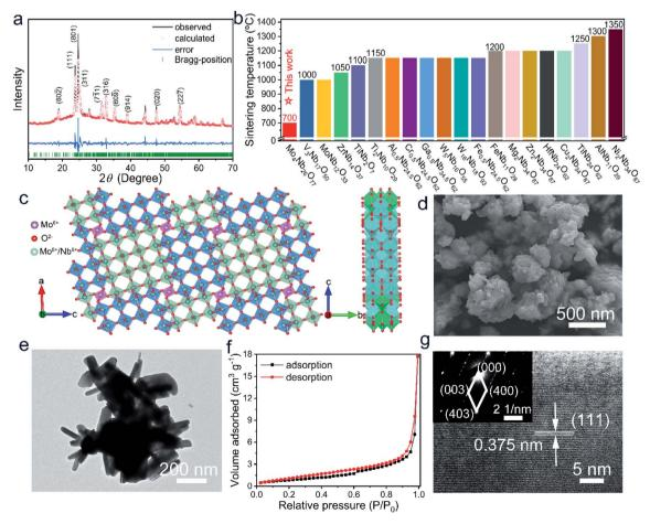
Fig. 1 Physico-chemical characterization studies of  $Mo_4Nb_{26}O_{77}$ . (a) Rietveld-refined XRD pattern. (b) Sintering temperature of  $Mo_4Nb_{26}O_{77}$ . from the solid-state reaction compared with other niobates. (c) Crystal structure viewed from different directions. (d) FESEM and (e) TEM images. (f) N<sub>2</sub> adsorption-desorption isotherms. (g) HRTEM image (inset: SAED pattern).
