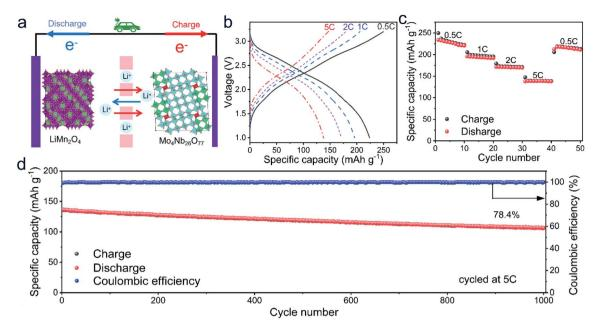
Fig. 3 Electrochemical properties of the  $LiMn_2O_4/Mo_4Nb_26O_{77}$  full cell. (a) Schematic illustration of a full cell. (b) GCD curves at various current rates. (c) Rate performance. (d) Long-term cyclability over 1000 cycles at 5C.
