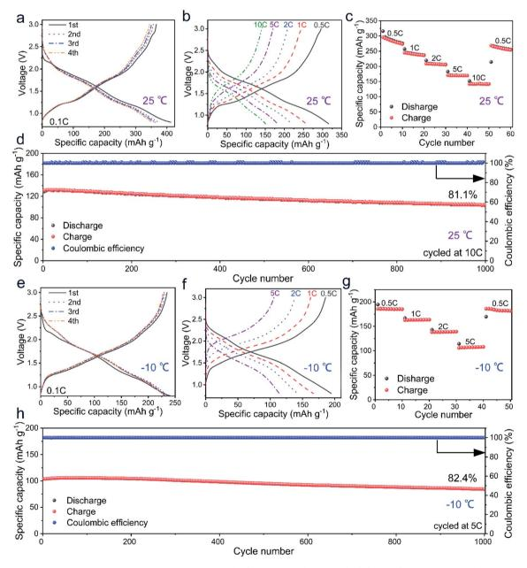
Fig. 2 Electrochemical characterization studies of the  $Mo_4Nb_{26}O_{77}/Li$  half cell at 25 and  $-10\,^{\circ}$ C. (a and e) First four-cycle GCD curves at 0.1C. (b and f) GCD curves at various current rates. (c and g) Rate performance. (d and h) Long-term cyclability over 1000 cycles.
