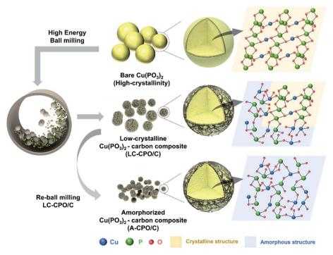
Fig. 1 Scheme of the fabrication process from bare Cu(PO<sub>3</sub>)<sub>2</sub> to LC-CPO/C and A-CPO/C with approximate material structure images.
