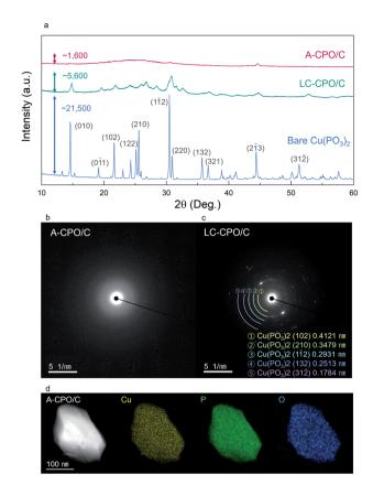
Fig. 2 (a) Comparing XRD patterns and the maximum intensities of bare Cu(PO<sub>3</sub>)<sub>2</sub>, LC-CPO/C and A-CPO/C. TEM SAED patterns of (b) A-CPO/C, (c) LC-CPO/C, (d) EDS elemental mapping (Cu: yellow, P: green, O: blue) of A-CPO/C.
