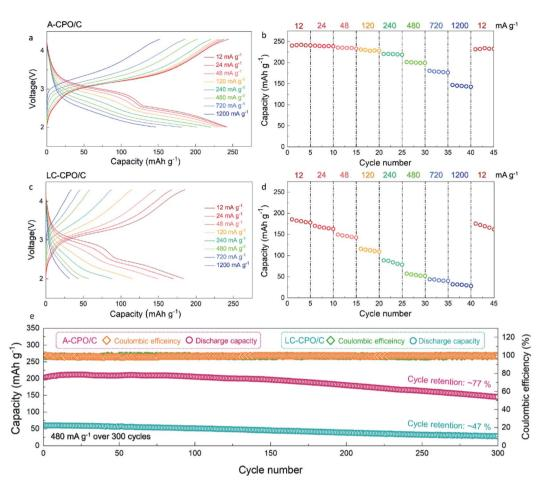
Fig. 4 Power capability of (a) A-CPO/C and (c) LC-CPO/C at various current densities in the voltage range of 2.0-4.3 V. Rate capability of (b) A-CPO/C and (d) LC-CPO/C. (e) Cycle performances of A-CPO/C and LC-CPO/C for 300 cycles at a current density of 480 mA g<sup>-1</sup> after an initial cycle at 30 mA g<sup>-1</sup>
