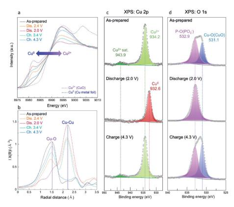
Fig. 6 Ex situ measurements of A-CPO/C electrodes for (a) XANES spectra, (b) EXAFS spectra, (c) XPS Cu 2p spectra, and (d) XPS O 1s spectra.
