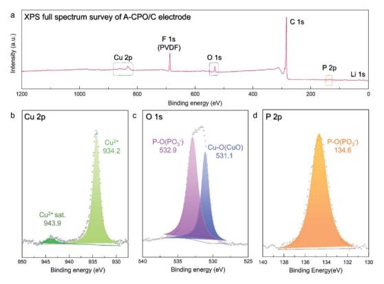
XPS spectra of A-CPO/C: (a) XPS full spectrum survey, (b) Cu 2p, (c) O 1s, and (d) P 2p.
