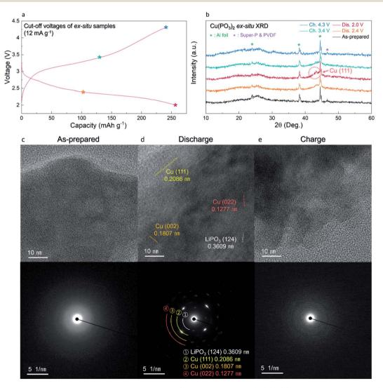
Fig. 5 (a) Cut-off voltage points of the *ex situ* samples on the charge/discharge curve of A-CPO/C. (b) *Ex situ* XRD patterns of A-CPO/C. HRTEM images with SAED patterns of (c) as-prepared, (d) discharged, and (e) charged A-CPO/C.
