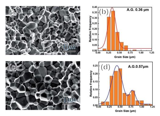
Fig. 3 (a and c) SEM images of freshly fractured surfaces of Co<sub>0.94</sub>Ni<sub>0.06</sub>SbS and Co<sub>0.94</sub>Ni<sub>0.06</sub>SbSo<sub>0.96</sub>Te<sub>0.04</sub>, respectively; (b and d) their corresponding grain-size distribution analysis.
