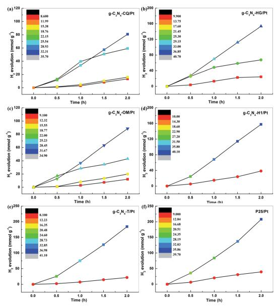
Fig. 3 The general phenomenon for STAP  $H_2$  evolution kinetics. The  $H_2$  evolution yield correlated with system temperature elevation at a variable time under simulated solar light irradiation for the photocatalyst of (a)  $g-C_3N_4-CQ/Pt$ , (b)  $g-C_3N_4-HG/Pt$ , (c)  $g-C_3N_4-DQ/Pt$ , (d)  $g-C_3N_4-DQ/Pt$ , (e)  $g-C_3N_4-DQ/Pt$ , (f) P25 (TiO<sub>2</sub>)/Pt. Inset: color scale bar representing system temperature elevation. Photocatalyst loading, 10 mg.
