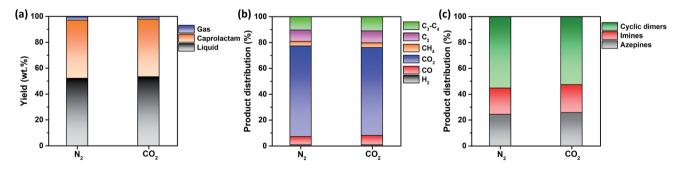
Fig. 3 (a) Yields of gaseous and liquid products, and caprolactam produced from the non-catalytic thermal conversion of FNW at 500  $^{\circ}$ C under  $N_2$  and  $CO_2$  environments; (b) distribution of gaseous products; (c) distribution of liquid products.
