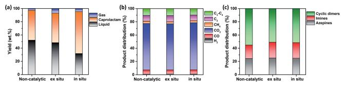
Fig. 6 (a) Yields of gaseous and liquid products, and caprolactam produced from the thermocatalytic conversion of FNW at 500  $^{\circ}$ C under an N<sub>2</sub> environment using SSWC-N2 in different catalyst configurations; (b) distribution of gaseous products; (c) distribution of liquid products.
