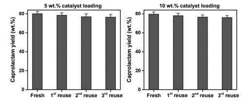
Fig. 9 Reusability of the spent SSWC-CO<sub>2</sub> catalyst with different catalyst loadings for the thermocatalytic conversion of FNW at 500 °C under a CO2 environment.
