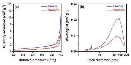
Fig. 4 (a) N<sub>2</sub> adsorption–desorption isotherm; (b) pore size distribution under N<sub>2</sub> physisorption for SSWC-N<sub>2</sub> and SSWC-CO<sub>2</sub>.
