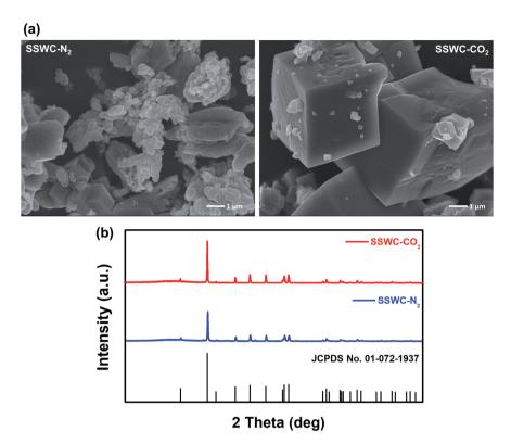
Fig. 5 (a) Scanning electron microscopy (SEM) images of SSWC- $N_2$  and SSWC- $CO_2$  (SEM images with a magnification of 5  $\mu$ m are given in Fig. S7†); (b) XRD patterns of SSWC- $N_2$  and SSWC- $CO_2$ .
