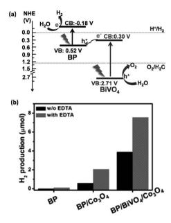
Fig. 10 (a) Schematic presentation of BP/BiVO $_4$  composite based Z-scheme photocatalyst for visible and NIR radiation (>420 nm) induced overall water splitting. (b)  $\rm H_2$  evolved by different catalysts with and without  $\rm Co_3O_4$  co-catalyst and EDTA sacrificial agent under >420 nm light irradiation. Reproduced with permission from ref. 118, © 2018 Wiley-VCH Verlag GmbH & Co. KGaA, Weinheim.
