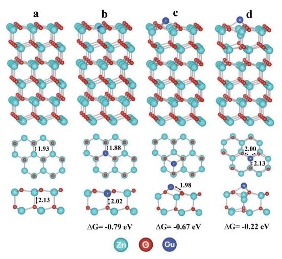
Fig. 4 The optimized structures of (a) pure ZnO, (b) doped  $Cu_1@ZnO$ , and (c and d) supported  $Cu_1/ZnO$ . The formation Gibbs free energies of doped and supported  $Cu_1$  are calculated at 298.15 K and 1 atm. The blue, cyan, and red spheres represent  $Cu_1$ ,  $Cu_2/2nO$ , and  $Cu_3/2nO$ , respectively.
