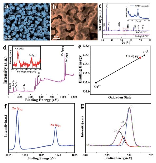
Fig. 1 The FESEM images of (a) ZnO/GPET and (b) Cu<sub>1</sub>-ZnO/GPET. (c) The XRD patterns of ZnO/GPET and Cu<sub>1</sub>-ZnO/GPET nanomaterials, where inset shows GPET substrate peaks. (d) XPS spectra for  $Cu_1$ -ZnO/GPET films and the inset shows Cu 2p peaks. (e) The binding energy of Cu  $2p_{3/2}$  with +2 and +1 oxidation states, respectively. (f and g) High resolution XPS scan of Zn 2p and O 1s for  $Cu_1$ -ZnO/GPET.
