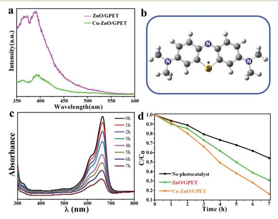
Fig. 3 (a) PL spectra of the Cu<sub>1</sub>-ZnO/GPET composite. (b) Schematic structure of MB<sup>+</sup> cation (optimized by using PBE/6-31G with Gaussian program). (c) Temporal evolution of the UV-vis absorption spectrum in accord with MB of  $Cu_1$ -ZnO/GPET. (d) Photodegradation rate of MB stimulated by UV of samples.
