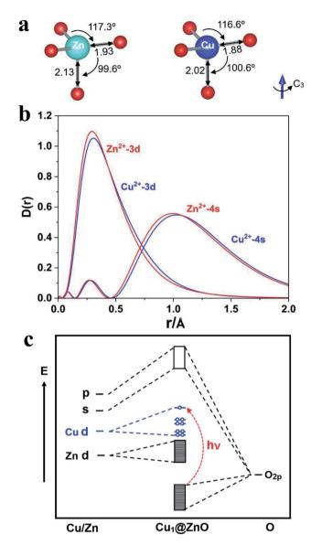
Fig. 6 (a) The local  $C_{3v}$  ligand field of ZnO and doped Cu<sub>1</sub>@ZnO surface in crystal (color code: Cu-blue, O-red, Zn-green). (b) The radial distribution probability density  $(D(r) = r^2R(r)^2)$  of atomic orbitals (AOs) of Zn(II) and Cu(II); (c) schematic energy levels of the Cu<sub>1</sub>@ZnO singleatom catalyst.
