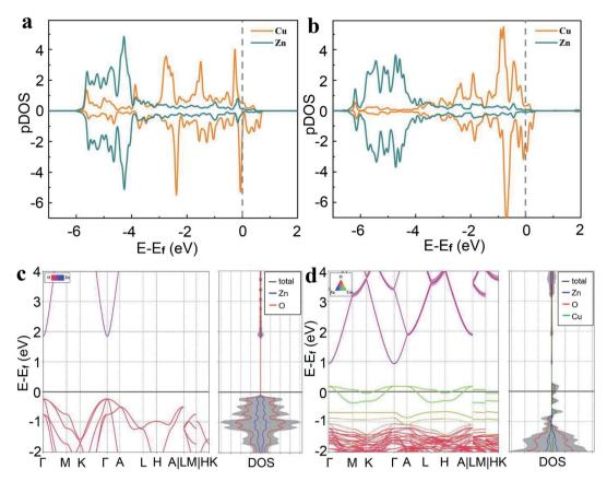
Fig. 5 Projected density of state (pDOS) of surface Zn and Cu atoms in (a) doped Cu<sub>1</sub>@ZnO model (Fig. 4b), and (b) supported Cu<sub>1</sub>/ZnO model (Fig. 4c). Band structure of (c) pure ZnO and (d) doped Cu<sub>1</sub>@ZnO in which one Zn atom in the  $2 \times 2 \times 2$  supercell of ZnO is replaced by one Cu atom
