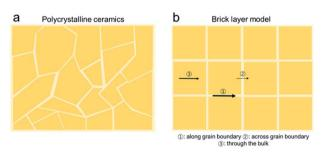
Fig. 3 A schematic showing (a) the cross section of a polycrystalline solid typically modelled using (b) the brick-layer model. The arrows indicate the different transport processes (1) rapid "diffusion pipes" along the grain boundary core, (2) across the grain boundary and (3) mass transport through an individual grain. The line thickness is proportional to the conductance of the associated process. 42
