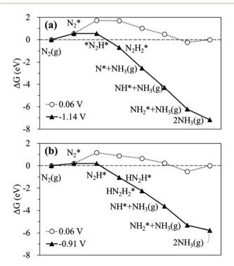
Fig. 3 Calculated free energy profiles at equilibrium (O) and limiting ( $\triangle$ ) potentials for the N<sub>2</sub>RR on (a) the Ru SAC and (b) the homo-Ru<sub>2</sub> DAC via the most favourable pathway.
