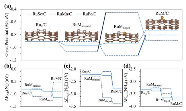
Fig. 8 Contribution of strain, dopant and configurational effects to the (a) onset potential, and adsorption energy of (b) N<sub>2</sub>, (c) N<sub>2</sub>H, and (d) NH<sub>2</sub> of the  $N_2RR$  on the hetero-RuM DACs. In (a), the bold solid lines indicate the change in the limiting step from  $[N_2* + (H^+ + e^-) \rightarrow N_2H^*]$  to  $[NH_2* + (H^+ + e^-) \rightarrow N_2H^*]$  $(H^+ + e^-) \rightarrow NH_3(g)].$
