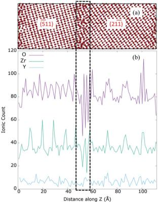
Fig. 6 (a) 8YSZ GB system.  $O^{2-}$ ,  $Zr^{4+}$  and  $Y^{3+}$  are represented by red, blue and grey spheres, respectively. (b) Calculated ionic count as a function of distance perpendicular to the GB core. The dotted box in (a) and (b) represent the GB core.
