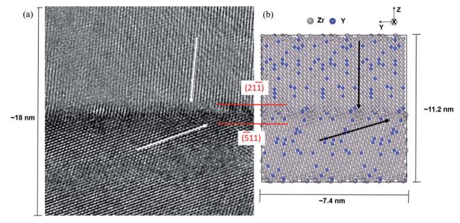
Fig. 3 (a) The TEM image of a mixed GB formed by (-511) and (21-1) orientated grains, with a misorientation angle of 52° and (b) the computational model representing the same mixed GB, prepared by amorphization and recrystallization method.
