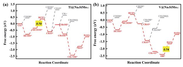
Calculated free energy diagrams for the electrochemical CO<sub>2</sub>RR on (a) Ti and (b) V@Na<sub>4</sub>SiMo<sub>12</sub>.
