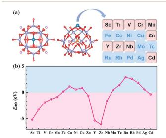
Fig. 3 (a) Schematic illustration of the transition metals anchored on  $Na_4SiMo_{12}$ . (b) The adsorption energies of transition metal atoms anchored on  $Na_4SiMo_{12}$ .
