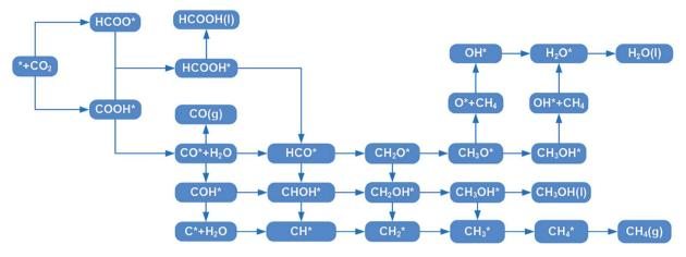
Scheme 1 All considered reaction pathways for CO<sub>2</sub> reduction on TM@Na<sub>4</sub>SiMo<sub>12</sub>
