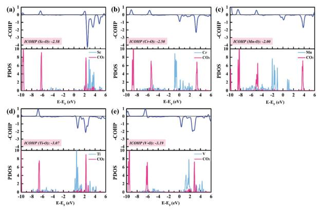
The PDOSs and COHPs of  $CO_2$  on  $TM@Na_4SiMo_{12}$  (TM = Sc, Cr, Mn, Ti and V).
