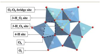
Fig. 1 Structure of an  $\alpha$ -Keggin type polyoxometalate.
