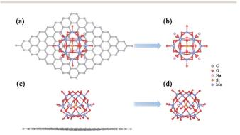
Fig. 2 Top views (a and b) and side views (c and d) of the most stable structures of  $Na_4SiMo_{12}$  loaded with or without graphene.
