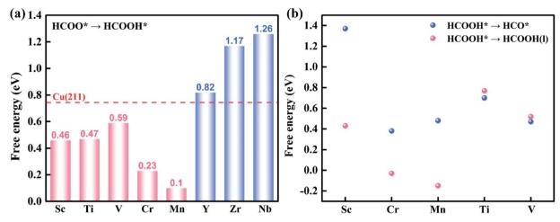
Fig. 5 (a) The  $\Delta G$  of HCOO\* + e $^-$  + H $^+$   $\rightarrow$  HCOOH\* on TM@Na<sub>4</sub>SiMo<sub>12</sub> (TM = Sc, Ti, V, Cr, Mn, Y, Zr and Nb). The screening criterion for catalytic activity is set to  $\Delta G < 0.74$  eV (red dashed line). (b) The  $\Delta G$  for HCOOH\* hydrogenation (HCOOH\* + e<sup>-</sup> + H<sup>+</sup>  $\rightarrow$  HCO\* + H<sub>2</sub>O (l)) and desorption  $(HCOOH^* \rightarrow HCOOH (I) + *)$  on  $TM@Na_4SiMo_{12}$  (TM = Sc, Cr, Mn, Ti and V).
