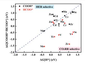
Fig. 4 Free energy change ( $\Delta G$ ) of the first protonation step in the CO<sub>2</sub>RR and HER on TM@Na<sub>4</sub>SiMo<sub>12</sub>.
