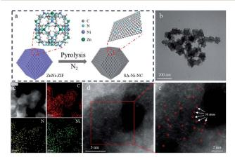
Fig. 1 Schematic illustrations of the preparation and structural characterization of SA-Ni-NC. (a) The synthesis process of SA-Ni-NC. (b) TEM, (c) HAADF-STEM and corresponding C, N, Ni elemental mapping, and (d, e) magnified HAADF-STEM images of SA-Ni-NC.
