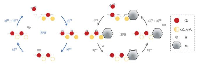
Fig. 1 Schematic diagram of the water electrolysis reaction via the two-phase boundary (left) and three-phase boundary (right) mechanisms.
