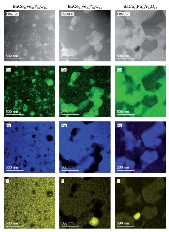
Fig. 4 STEM-HAADF images with EDXS elemental maps for selected cations of composite ceramics obtained from precursors of  $BaCe_{0.2}$ - $Fe_{0.6}Y_{0.2}O_{3-\delta}$  (left column),  $BaCe_{0.4}Fe_{0.4}Y_{0.2}O_{3-\delta}$  (in the middle) and  $BaCe_{0.6}Fe_{0.2}Y_{0.2}O_{3-\delta}$  (right column) by spark plasma sintering (conditions given in Table S6†). The bright grains in the Y maps are occasional Y-rich precipitates.
