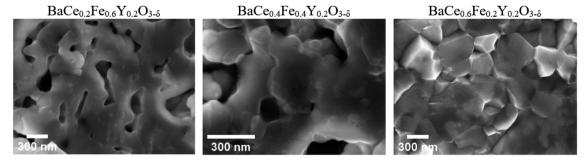
Fig. 3 SEM images of BaCe<sub>0.2</sub>Fe<sub>0.6</sub>Y<sub>0.2</sub>O<sub>3-δ</sub>, BaCe<sub>0.4</sub>Fe<sub>0.4</sub>Y<sub>0.2</sub>O<sub>3-δ</sub> and BaCe<sub>0.6</sub>Fe<sub>0.2</sub>Y<sub>0.2</sub>O<sub>3-δ</sub> composite ceramics (SPS sintering, Table S6†) recorded along fracture planes with an in-lens secondary electron detector.
