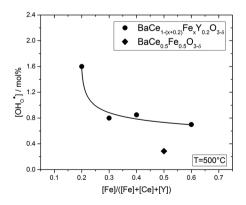
Fig. 6 Proton concentration of composites obtained from precursors of BaCe  $_{0.5}$  Fe  $_{0.5}$  O  $_{3-\delta}$  (open symbol) and BaCe  $_{1-(\text{x}+0.2)}$  Fe  $_{\text{x}}$  Y  $_{0.2}$  O  $_{3-\delta}$  (0.2  $\leq x \leq$  0.6) (closed symbols) as a function of Fe content for  $T = 500 \,^{\circ}\text{C}$ . The line connecting the circles is a guide to the eye.
