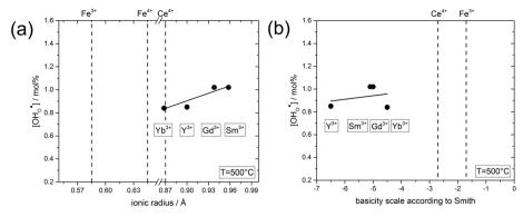
Fig. 7 (a) Proton concentration at 500 °C of composites obtained from precursors of BaCe<sub>0.4</sub>Fe<sub>0.4</sub>B<sub>0.2</sub>O<sub>3- $\delta$ </sub> (B = Yb, Y, Gd or Sm) as a function of the ionic radius<sup>29</sup> of B. (b) Proton concentration at 500 °C of composites obtained from precursors of BaCe<sub>0.4</sub>Fe<sub>0.4</sub>B<sub>0.2</sub>O<sub>3- $\delta$ </sub> (B = Yb, Y, Gd or Sm) as a function of the basicity<sup>39</sup> of the binary oxides of B.
