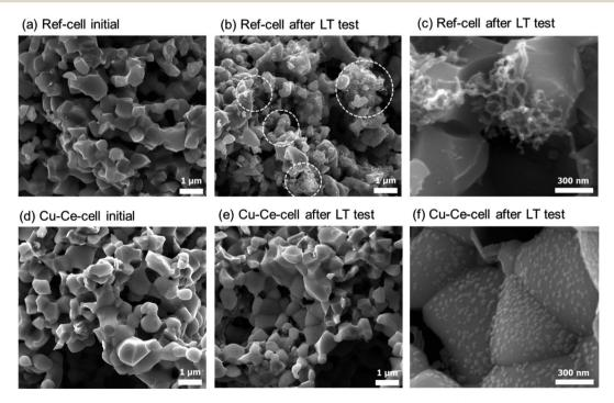
Fig. 8 SEM images of as-prepared and tested cells. SEM images of as-prepared cells: (a) ref-cell and (d) Cu-Ce-cell. SEM images of (b and c) ref-cell and (e and f) Cu-Ce-cell after the long-term testing procedure demonstrated in Fig. 6.
