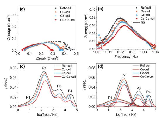
Fig. 5 Electrochemical impedance analysis of ISRB-TF-SOFCs. EIS data from the four TF-SOFCs in ISRB mode at 600 °C with an SCR of 3 at 0.2 A cm<sup>-2</sup>: (a) Nyquist plots; (b) Bode plots; (c) DRT results; and (d) DRT fitting plots demonstrating distinct peaks for each TF-SOFC (note that the P4 peak of Cu-cell overlaps with the P4 peak of Ce-cell in (d)).
