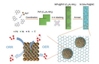
Fig. 1 Schematic illustration showing the formation pathway of Ni SAs-PdaNC.
