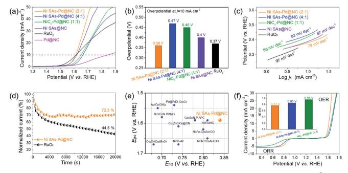
Fig. 5 (a) OER polarization curves recorded in  $O_2$ -saturated 0.1 M KOH. (b) Bar plots of overpotentials obtained at 10 mA cm $^{-2}$ . (c) Corresponding Tafel plots. (d) Chronoamperometric curve recorded at 1.6 V. (e) Plot of comparison of catalysts from references. (f) Overall polarization curves.
