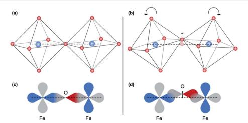
Fig. 12 Schematic representation of the effect of the Fe-O-Fe bond angle on the O 2p and Fe 3d orbital overlap. The arrow indicates the change in position of the bridging oxygen.
