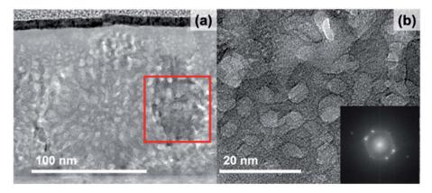
Fig. 3 Bright-field TEM images of an amorphous-grown STF35 thin film annealed at 400  $^{\circ}$ C in  $\sim$ 0.2 atm UHP O<sub>2</sub> and  $\sim$ 0.8 atm UHP Ar for 20 min at low (a) and high (b) magnification and an FFT (b, inset) of the region outlined by the red box.
