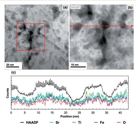
Fig. 5 HAADF STEM image of an amorphous-grown STF35 thin film annealed at  $400 \,^{\circ}$ C in  $\sim$ 0.2 atm UHP O<sub>2</sub> and  $\sim$ 0.8 atm UHP Ar for 20 min (a), the EDS mapping region (outlined in red (a)), and line scan path (b), and the HAADF intensity and Sr, Ti, Fe, and O intensities from the EDS line scan (c).
