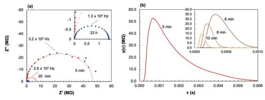
Fig. 9 Nyquist plot (a) and DRT spectra (b) of select impedance spectra collected during in situ crystallization at 400  $^{\circ}$ C in  $\sim$ 0.2 atm UHP O<sub>2</sub> and  $\sim$ 0.8 atm UHP Ar.
