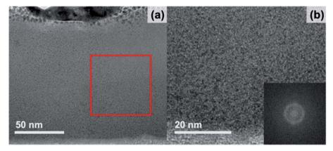
Fig. 2 Bright-field TEM images of an amorphous-grown STF35 thin film annealed at 400 °C in  $\sim$ 0.2 atm UHP O<sub>2</sub> and  $\sim$ 0.8 atm UHP Ar for 5 min at low (a) and high (b) magnification and an FFT (b, inset) of the region outlined by the red box.
