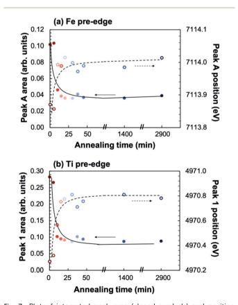
Fig. 7 Plot of integrated peak area (closed symbols) and position (open symbols) of pre-edge peaks A at the Fe K-edge (a) and 1 at the Ti K-edge (b) as a function of annealing time at 400 °C in ~0.2 atm UHP  $O_2$  and  $\sim 0.8$  atm UHP Ar.
