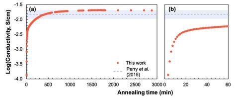
Fig. 10 Plot of conductivity over the full annealing period (a) and over the first hour (b) at 400 °C in  $\sim$ 0.2 atm UHP O<sub>2</sub> and  $\sim$ 0.8 atm UHP Ar; dashed line shows the conductivity and conservative uncertainty estimate (shaded blue) of a crystalline-grown STF35 thin film<sup>26</sup> under the same conditions
