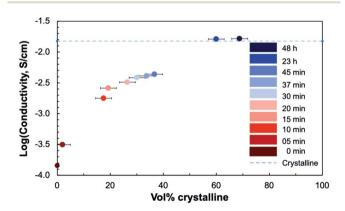
Fig. 11 Plot of the logarithmic in-plane total conductivity at 400 °C in  $\sim$ 0.2 atm UHP O<sub>2</sub> and  $\sim$ 0.8 atm UHP Ar as a function of crystalline volume percent of crystallizing STF35 thin films. The conductivity of a crystalline-grown STF35 thin film, from ref. 26, measured under the same conditions is marked by the dashed line
