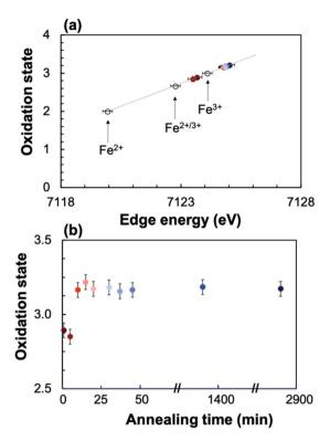
Fig. 8 The linear trend between oxidation state and edge energy for FeO (Fe $^{2+}$ ), Fe $_3O_4$  (Fe $^{2+/3+}$ ), and Fe $_2O_3$  (Fe $^{3+}$ ) was interpolated/extrapolated to calculate the oxidation state of each annealed STF35 sample from the edge position (a). The calculated oxidation state for each STF35 sample is plotted as a function of annealing time at 400  $^{\circ}$ C in  $\sim\!0.2$  atm UHP O $_2$  and  $\sim\!0.8$  atm UHP Ar (b).
