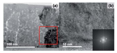
Fig. 4 Bright-field TEM images of an amorphous-grown STF35 thin film annealed at 400 °C in  $\sim$ 0.2 atm UHP O<sub>2</sub> and  $\sim$ 0.8 atm UHP Ar for 23 h at low (a) and high (b) magnification and an FFT (b, inset) of the region outlined by the red box.
