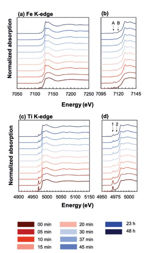
Fig. 6 Plot of normalized XANES spectra of annealed, amorphous-grown STF35 thin films at the Fe (a and b) and Ti (c and d) K-edges. Two preedge features are labeled with A and B at the Fe K-edge (c) and with 1 and 2 at the Ti K-edge (d). Legend indicates annealing times at 400  $^{\circ}$ C in  $\sim$ 0.2 atm UHP O<sub>2</sub> and  $\sim$ 0.8 atm UHP Ar.
