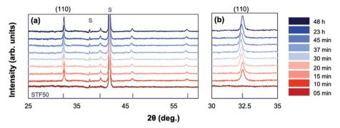
Fig. 1 Background-subtracted X-ray diffraction patterns for amorphous-grown STF35 thin films annealed for a series of times along a 400 °C isothermal hold in  $\sim$ 0.2 atm UHP  $O_2$  and  $\sim$ 0.8 atm UHP Ar. Substrate peaks are marked with an S. Peak positions for STF50 are marked with vertical bars for reference (PDF#97-018-4374).
