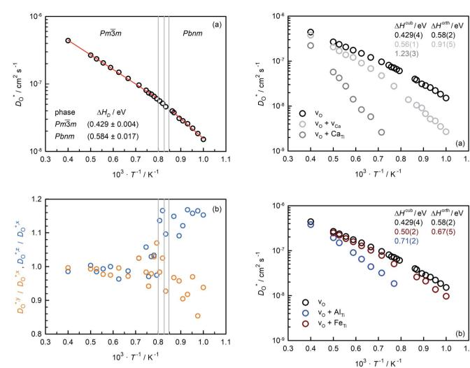
Fig. 4 Oxygen tracer diffusion coefficients obtained for a  $CaTiO_3$  system containing only oxygen vacancies as a function of inverse temperature: (a) total values, (b) ratios of axis-specific values. Error bars are smaller than the symbol size.
