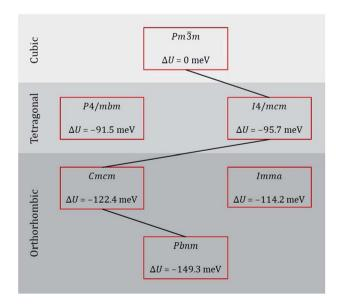
Fig. 2 Lattice energy U of various phases of  $CaTiO_3$  relative to that of the ideal cubic phase. The black line indicates the probable sequence of transitions.
