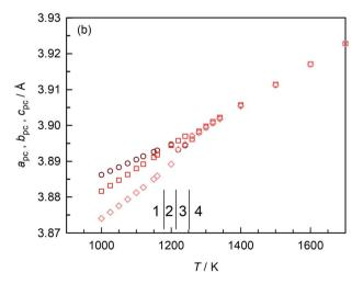
Fig. 3 Pseudo-cubic lattice parameters obtained as a function of temperature: (a) stoichiometric CaTiO<sub>3</sub>; (b) oxygen-deficient CaTiO<sub>3</sub>.
