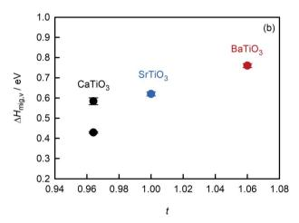
Fig. 7 Comparison of data for titanate perovskites obtained from MD simulations: (a) oxygen-vacancy diffusivities versus inverse temperature, (b) activation enthalpy for oxygen-vacancy migration versus Goldschmidt tolerance factor. CaTiO<sub>3</sub> (this study), SrTiO<sub>3</sub> (Waldow and De Souza<sup>56</sup>), BaTiO<sub>3</sub> (Kaub et al.<sup>50</sup>)
