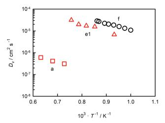
Fig. 6 Oxygen-vacancy diffusion coefficients in  $CaTiO_3$  as a function of inverse temperature: a (George and Grace<sup>35</sup>), e1 (Bak *et al.*<sup>39</sup>), f (this study).
