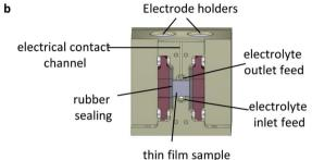
Fig. 4 Operando reactor cell for surface sensitive GIXAS measurements. (a) Trimetric view of the cell and GIXAS geometry used during measurements, where the grazing incident X-rays enter through a Mylar foil covered side window (PIPS denotes a passivated implanted planar silicon detector), (b) cross sectional internal view.
