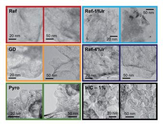
Fig. 2 TEM images of the FeNC catalyst Ref as well as the iridium modified FeNC catalysts and Ir/C.
