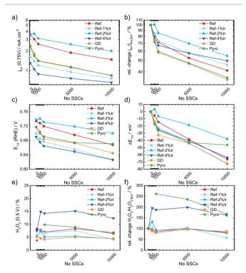
Fig. 9 Change in kinetic current density (a) absolute scale, (b) relative scale, half wave potential (c) absolute value, (d)  $\Delta E_{1/2}$  and hydrogen peroxide formation (e) absolute and (f) relative as a function of the number of SSCs.
