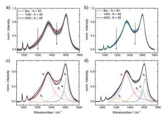
Fig. 11 Averaged spectra including standard deviation for (a) Ref and (b) Ref-4% Ir catalysts and fitted spectra of (c) Ref and (d) Ref-4% Ir catalysts. Spectra were obtained BoT, after 1000 and 5000 SSCs at RT in the *in situ* Raman setup described in the experimental section.
