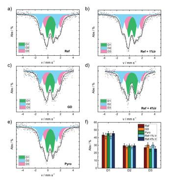
Fig. 5 Mössbauer spectra of the catalysts as indicated (a) Ref, (b) Ref+1% Ir, (c) GD, (d) Ref+4% Ir, (e) Pyro and (f) comparison of the relative absorption areas for the different catalysts.
