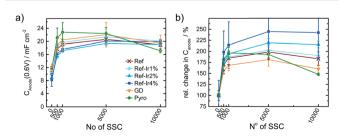
Fig. 8 (a) Change in capacitance and relative change in capacitance as a function of the number of SSC cycles applied to the catalysts. Values extracted from CV measurements in  $\rm N_2$  saturated 0.1 M  $\rm H_2SO_4$ .
