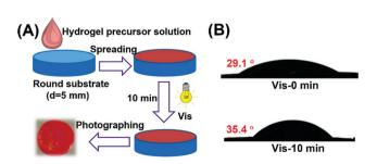
Fig. 4 (A) Schematic for the fabrication process of hydrogel coatings. (B) Pictures of water droplets on the coating of hydrogel precursor solution and the hydrogel coating with 10 min irradiation by marking the corresponding contact angles values.
