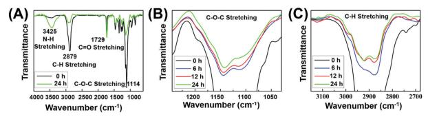
Fig. 2 IR spectra of (A) P(EMA-SS-PEG) and its hydrogel with 24 h irradiation; (B) C-O-C stretching and (C) C-H stretching of P(EMA-SS-PEG) (0 h) and its hydrogels with irradiation of 6, 12 and 24 h. The peak intensity of C=O stretching was constant and served as a reference value.
