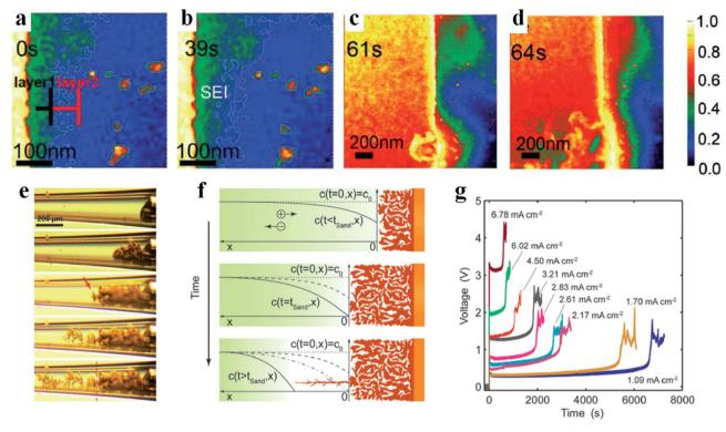
Fig. 2 Formation of SEIs and lithium dendrites. (a-d) Time sequential high-angle annular dark-field STEM (HAADF-STEM) images of SEIs. Reproduced with permission.<sup>46</sup> Copyright 2019, Wiley-VCH. (e) In situ optical photograph of lithium growth. (f) Theoretical interpretation of lithium deposition during concentration polarization. (g) Voltage responses under various current densities. Reproduced with permission.<sup>48</sup> Copyright 2016, The Royal Society of Chemistry.
