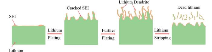
Fig. 1 Schematic drawing illustrating the formation process of SEIs and lithium dendrites during lithium battery cycling
