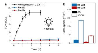
Fig. 3 Photocatalytic  $CO_2$  reduction performance. (a) TON(CO) vs. time plot for MOF samples, including the homogeneous reference (black trace). (b) Product evolution rates averaged over the first two irradiation hours. Standard conditions: MOF sample (1.5 mg) suspended in MeCN (4 mL) and deionised  $H_2O$  (0.12 mL) with BIH (225 mg), room temperature, continuous >430 nm irradiation.
