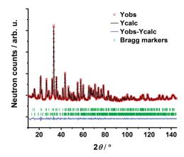
Fig. 1 Rietveld refinement of  $Cs_3MoO_4D$  based on powder neutron diffraction. Bragg markers:  $Cs_3MoO_4D$  (top) (90.3(10) wt%); CsD (bottom) (9.7(1) wt%).  $R_p = 1.18\%$ ,  $R_{wp} = 1.57\%$ ,  $R_{exp} = 0.83\%$ ,  $R_{Bragg} = 1.60\%$ ,  $\chi^2 = 3.59$ .
