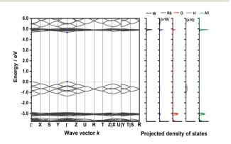
Fig. 5 Electronic band structure of  $Rb_3WO_4H$  and projected density of states (DFT-PBE0). The band paths in the reciprocal space have been determined by the Seek-path webservice.<sup>45</sup> The DOS of Rb and H are enhanced by a factor of ten for better visibility.
