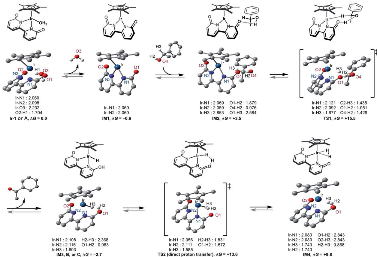
Fig. 5 Geometry and energy changes of the proposed pathway at the CAM-B3LYP + GD3 level of theory using SDD and 6-31++G\*\* basis sets for Ir and other atoms, respectively. Solvent effect (H<sub>2</sub>O) by IEFPCM method; Gibbs free energies in kcal mol<sup>-1</sup> at  $T = 353.15$  K.
