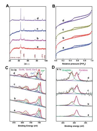
Fig. 2 (A) Powder XRD patterns, (B)  $N_2$ -adsorption—desorption isotherms, (C) Co 2p spectra and (D) N 1s spectra. In the figures, a, b, c, and d represent Co@C—N(600), Co@C—N(700), Co@C—N(800), and Co@C—N(900), respectively.
