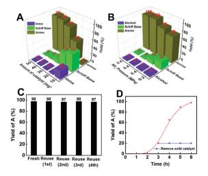
Fig. 3 (A) Effect of the catalyst amount, (B) effect of NH $_3$  pressure, (C) reusability of Co@C–N(800), and (D) time–yield plots for reductive amination of cyclohexanone with Co@C–N(800) (red line) or removing Co@C–N(800) after 3 h (blue line). Reaction conditions: cyclohexanone, 1 mmol; methanol, 3 mL; 35 °C; 6 h; Co@C–N(800), 50 mg (29.2 mol% Co); total pressure of NH $_3$  and H $_2$  was 2 MPa and 1.4 MPa H $_2$  and 0.6 MPa NH $_3$  in part D.
