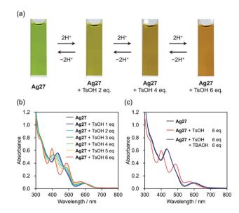
Fig. 2 (a) Color change of Ag27 after addition of 0-6 equivalents of p-toluenesulfonic acid (TsOH) and tetra-n-butylammonium (TBAOH) in acetonitrile. UV-Vis spectra of (b) Ag27 before and after addition of 0-6 equivalents of TsOH and (c) Ag27 before and after addition of 6-6 equivalents of TsOH and TBAOH in acetonitrile (10-6 µM, 1-6 cm cell).
