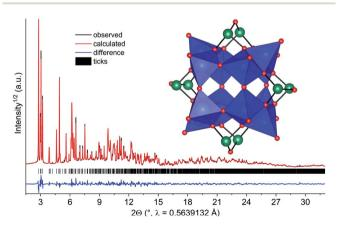
Fig. 7 Difference plot of the final Rietveld refinement for [Ni(en)<sub>3</sub>]<sub>2</sub>[-As<sub>8</sub>V<sub>12</sub>O<sub>40</sub>(H<sub>2</sub>O)]·4H<sub>2</sub>O with a final  $R_{wp}$  of 4.7% and  $R_{Bragg}=3.7\%$ . The inset shows the polyhedral representation of the cluster anion in the structure of **2**. Note: the H<sub>2</sub>O molecule in the cavity of the cluster is not displayed. Blue: VO<sub>5</sub> polyhedra; green: As; red: O.
