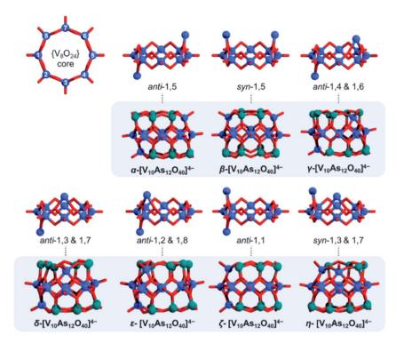
Fig. 13 Enumeration of the eight V centres in the  $\{V_8O_{24}\}$  cores deriving from the  $[V_8As_{16}O_{40}]$  structure (top left), followed by the depiction of substitution patterns and the respective  $[V_{10}As_{12}O_{40}]^{4-}$  isomers positioned in the shaded box areas colour code: V = blue, O = red, and As = green spheres.
