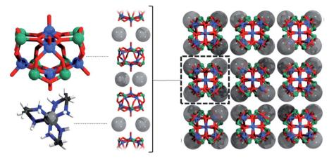
Fig. 3 Ball and stick representation of an individual  $[V_6As_8O_{26}]^{4-}$  polyanion and the  $[Ni(en)_3]^{2+}$  dications (left), followed by their hierarchical packing from one (middle) to three dimensions (right). Colour code: V = blue, O = red, As = green, N = dark blue, Ni = grey, C = black, H = whitespheres. For clarity,  $[Ni(en)_3]^{2+}$  in the middle and right figure are represented as transparent grey spheres.
