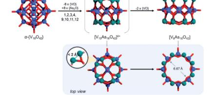
Fig. 12 Schematic juxtaposition of (a) substitution of four  $[VO]^{2+}$  sites in the central belt of  $\alpha$ - $\{V_{18}O_{42}\}$  leading to energetically unfavourable further  $2 \times [VO]^{2+}$  loss; (b) substitution of eight  $[VO]^{2+}$  sites of the two cupolaed in  $\alpha - (V_{18}O_{42})$  leading to geometrically favourable  $2 \times [VO]^{2+}$ loss. Colour code: V = blue, As = green, and O = red spheres.
