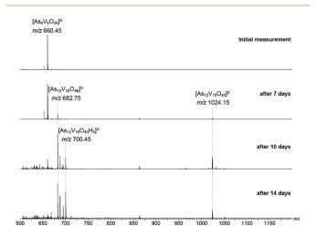
Fig. 8 ESI mass spectra of a 100  $\mu$ M solution of the parent compound in H<sub>2</sub>O recorded after different reaction times. The initial peak at m/z 660.45 decreases over days with a simultaneous increase of signals at m/z 682.75 and 1024.15 assigned to the -3 and -2 charge states of  $\{V_{10}As_{12}O_{40}\}$ . Peaks with additional oxygen/water molecules were also observed such as the ion at m/z 700.45.
