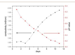
Fig. 6 Long-term investigation of the ionic conductivity and the pH value using an aqueous solution (8.26 mmol  $L^{-1} = 14.9 \text{ g L}^{-1}$ ) of the title compound. The lines are only guide for the eyes.
