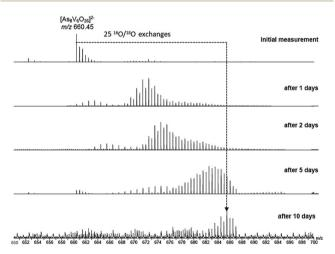
Fig. 9 ESI mass spectra of a 100  $\mu$ M solution of the parent cluster in H<sub>2</sub><sup>18</sup>O at different reaction times. After about 10 days, a mass shift corresponding to 25 O atom exchanges is achieved.
