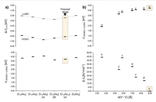
Fig. 14 Energy diagrams based on Tables S7 and S8,† showcasing (a) the α-spin HOMO and LUMO (top) and HOMO-LUMO gap (bottom) energies among different experimentally described As-POVs and the herein proposed  $\alpha$ -[ $V_{10}As_{12}O_{40}$ ]<sup>4-</sup> model; (b) HOMO-LUMO gap (top) and relative bonding energy in of the isomeric [ $V_{10}As_{12}O_{40}$ ]<sup>4-</sup> in comparison to the α-structure.
