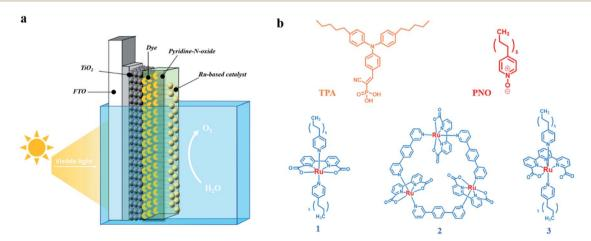
Fig. 2 (a) Schematic of the TiO2|dye|PNO|Cat photoanode employed for water oxidation. (b) Molecular structures of TPA dye, PNO and Rubased molecular water oxidation catalysts 1, 2 and 3 used in the study.
