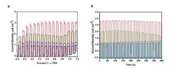
Fig. 5 (a) Photocurrent density–voltage (j-v) traces with 5 s light transients for TiO<sub>2</sub>|TPA|PNO (red), TiO<sub>2</sub>|TPA (green), TiO<sub>2</sub>|TPA|Nafion (blue) and TiO<sub>2</sub>|TPA|PMMA (black) scanned from -0.4 to 1.2 V vs. NHE with a scan rate of 1 mV s<sup>-1</sup> under 1 sun illumination in pH 7, 0.1 M phosphate buffer containing 0.1 M Na<sub>2</sub>SO<sub>3</sub>. (b) The time dependent photocurrent density (j-t) traces with 10 s light transients at 0.4 V vs. NHE.
