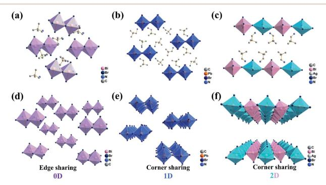
Fig. 1 Basic structures of  $(DPA)_4Bi_2Br_{10}$  (a),  $(DPA)_5Pb_2Br_9$  (b) and  $(DPA)_4AgBiBr_8$  (c) at low temperature. The dimension diagram of inorganic skeletons:  $(DPA)_4Bi_2Br_{10}$  (d),  $(DPA)_5Pb_2Br_9$  (e) and  $(DPA)_4AgBiBr_8$  (f). The hydrogen atoms are omitted for clarity.
