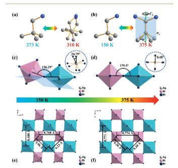
Fig. 3 Movement of the cation in  $(DPA)_5Pb_2Br_9$  (a) and  $(DPA)_4AgBiBr_8$  (b) in the low temperature and high temperature phase. Frontal and lateral (inset) torsion angles of a Bi-based octahedron with a Ag-based octahedron as the reference in  $(DPA)_4AgBiBr_8$  in the low temperature (c) and high temperature phase (d). Distance between metal atoms of  $(DPA)_4AgBiBr_8$  in the low temperature (e) and high temperature phase (f). The hydrogen atoms are omitted for clarity.
