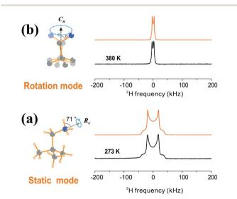
Fig. 4 Experimental (black) and simulated (orange) <sup>2</sup>H spectra of (DPA-d<sub>3</sub>)<sub>4</sub>AqBiBr<sub>8</sub>. This sample was synthesized by using N-deuterated DPA. The experimental spectra were acquired at 273 K (a) and 380 K (b). The simulated <sup>2</sup>H spectra were obtained based on the motion model on the left via Weblab (https://weblab2.mpip-mainz.mpg.de/ weblab66/weblab.html).
