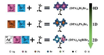
Scheme 1 Train of thought from a Bi-Br to Pb-Br to Ag-Bi-Br system based on DPA to realize lead-free hybrid double perovskite.
