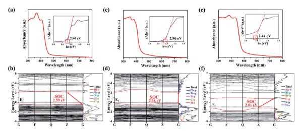
Fig. 6 The UV-vis absorption spectra, corresponding Tauc plots, and calculated energy band structure of  $(DPA)_4Bi_2Br_{10}$  (a) and (b),  $(DPA)_5Pb_2Br_9$  (c) and (d) and  $(DPA)_4AgBiBr_8$  (e) and (f) with spin-orbit coupling (SOC), and corresponding partial density of states (PDOS).
