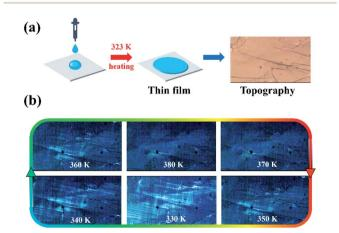
Fig. 5 (a) Preparation process and topography of a thin film. (b) Evolution of ferroelastic domains of (DPA)<sub>4</sub>AgBiBr<sub>8</sub> before and after phase-transition temperature (the contrast of the diagrams has been adjusted to observe the domain structures more clearly).
