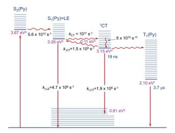
Fig. 7 Diagram of the excited state relaxation processes. <sup>a</sup>From 00energies of the absorption spectrum; bfrom 00-energies of the emission spectrum; <sup>c</sup>from the Stevens-Ban plot; <sup>d</sup>from b and c; <sup>e</sup>from  $d-E_{max(em)}$ ; fsee ref. 74.
