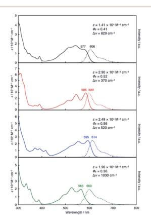
Fig. 3 UV-vis absorption (solid lines) and fluorescence spectra (dashed lines) of 10a (black), 11 (red), 12 (blue), and 13 (green) in toluene.
