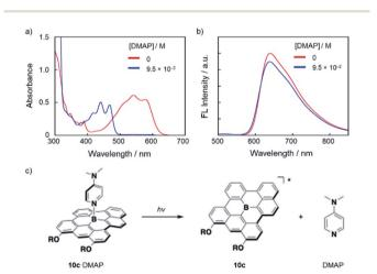
Fig. 5 (a) UV-vis absorption and (b) fluorescence ( $\lambda_{ex}=477$  nm) spectral changes upon addition of DMAP to a DMSO solution of  $10c \cdot 2.2 \times 10^{-5}$  M). (c) Schematic illustration of the photo-dissociation of  $10c \cdot 2.2 \times 10^{-5}$  MAP.
