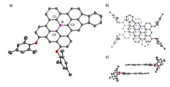
Fig. 2 (a) Crystal structure of 12 with thermal ellipsoids at 50% probability. Hydrogen atoms are omitted for clarity. (b) Top view and (c) side view of the  $\pi$ -stacked dimeric motif in the crystal packing of 12.
