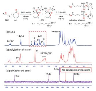
Fig. 1 One-pot synthesis of poly(ether-alt-ester) (Table 1, entry 1). <sup>1</sup>H NMR spectra of (a) crude intermediate product of SOE1, (b) poly(etheralt-ester), and (c) <sup>13</sup>C(<sup>1</sup>H) NMR spectrum of poly(ether-alt-ester) (400 MHz, C<sub>6</sub>D<sub>6</sub>, 25 °C).
