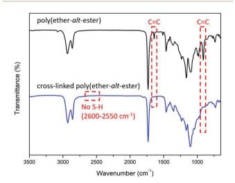
Fig. 2 Cross-linking of poly(ether-alt-ester) via thiolene reaction (top). FTIR spectra of poly(ether-alt-ester) and cross-linked poly(ether-alt-ester) (bottom).
