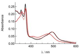
Fig. 4 (a) Changes in the electronic absorption spectrum of 2a in  $CH_3CN$  following irradiation,  $t_{\rm irr}=0-5$  min and (b) electronic absorption spectra of 2a before irradiation (solid red), following 30 min irradiation (dashed red), and 2b (black).
