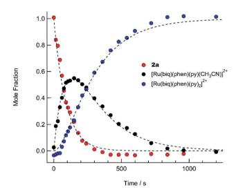
Fig. 7 Time dependent concentrations of 2a (red circles), cis- $[Ru(biq)(phen)(py)(CH<sub>3</sub>CN)]^{2+}$ black (I, circles),  $[Ru(biq)(phen)(py)_2]^{2+}$  following irradiation ( $\lambda_{irr} \ge 395$  nm) in pyridine from t = 0 to t = 1200 s. The dashed lines are least-squares fits to a consecutive reaction model with a system of equations describing the time-dependent concentration of each compound (see text).
