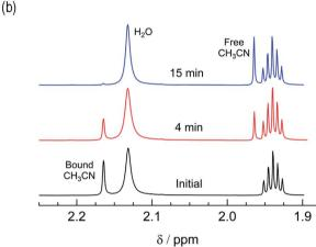
Fig. 3 Changes following the irradiation of 1a ( $\lambda_{irr} \ge 395$  nm) to the (a) electronic absorption spectrum in  $H_2O$ ,  $t_{irr}=0-30$  min, and (b)  $^1H$ NMR spectrum in CD<sub>3</sub>CN,  $t_{irr} = 0$ , 4, and 14 min.
