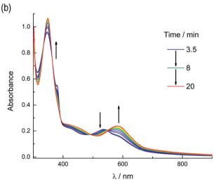
Changes following irradiation ( $\lambda_{irr} \ge 395$  nm) in the electronic absorption spectrum of 2a in pyridine from (a)  $t_{irr} = 0-2.5$  min and (b)  $t_{irr} = 3.5-20 \text{ min.}$
