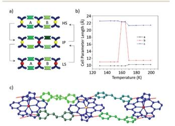
Fig. 6 (a) Schematic illustration of structural pathway between HS and LS phases, which both display AB supramolecular chain architectures and the IP, which contains four crystallographically distinct coformers. (b) Variation in unit cell lengths as a function of temperature. Unit cell angles are provided in the ESI† (c) view of the cocrystal in the IP showing long-range order of HS (yellow) and LS (red) sites along the supramolecular chains.
