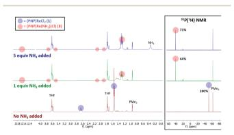
Fig. 2  $^{1}$ H and  $^{31}$ P{ $^{1}$ H} NMR spectra of 1 in THF- $d_{8}$  without NH $_{3}$ (bottom, maroon), with 1 equiv. NH<sub>3</sub> added (middle, green), and with 5 equiv. NH<sub>3</sub> added (top, blue). Spectroscopic yields reported vs. PMe<sub>3</sub> in a capillary
