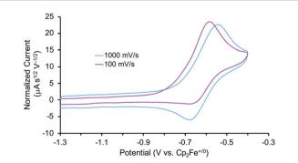
Fig. 3 Cyclic voltammogram of the first oxidation of 3 (0.2 mM) in  $0.2\,M\,NBu_4PF_6$  solution in THF under  $N_2$  using a glassy carbon working electrode, Pt wire auxiliary electrode, and Ag wire pseudoreference. Potentials referenced to  $Cp_2Fe^{+/0}$  after the experiments.
