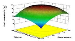
Fig. 5 Response surface diagram of cyclohexanone oxime conversion: (a) reaction temperature and catalyst amount, (b) reaction temperature and water consumption and (c) catalyst amount and water consumption.
