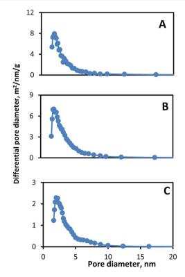
Fig. 2 Pore size distribution of mesoporous glass-ceramic frits (A, B and C) based on BJH analysis of nitrogen sorption isotherms.
