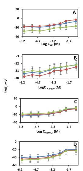
Fig. 5 Effect of different salts: KCl (A),  $Na_2SO_4$  (B),  $NaNO_3$  (C), and  $NBu_4ClO_4$  (D) on the potentiometric responses of reference electrodes constructed using nanoporous glass-ceramic composite. Green represents (frit A), blue (frit B), and red (frit C). Data are average of three separate but identical reference electrodes.
