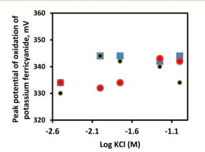
Fig. 6 Effect of concentration of KCl supporting electrolyte (3–100 mM) on the potential of three reference electrodes based on: mesoporous ceramic frit A (blue), mesoporous ceramic frit B (black), and commercially available free flow (red). Shown is the peak potential of the  $Fe(CN)_6^{4-}$  (0.1 mM) oxidation as determined from CVs.
