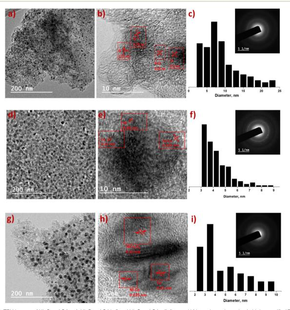
Fig. 2 HR-TEM images of  $Ni_6Co_4$ -AC (a-c),  $Ni_5Co_5$ -AC (d-f) and  $Ni_4Co_6$ -AC (g-i). (b, e and h) interplanar d-spacing in high magnified TEM; (c, f and i) particle size range of metals and SAED pattern.
