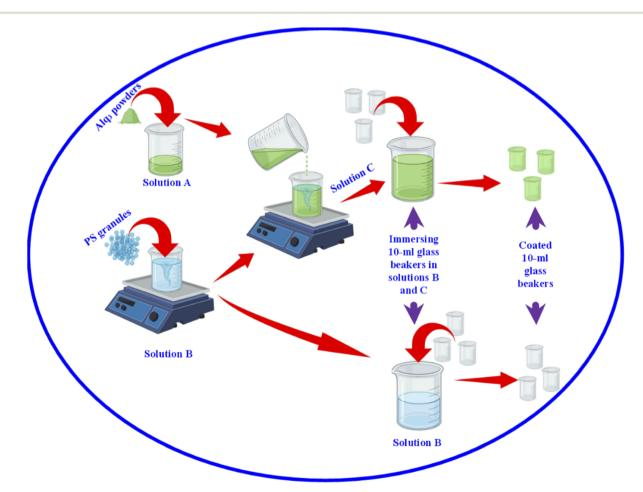
Fig. 2 Schematic diagram showing the fabrication of PS/Alg<sub>3</sub> as an antibacterial composite.
