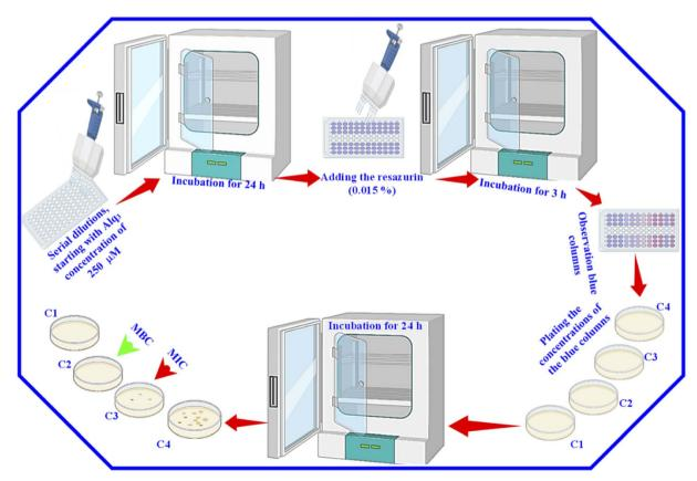
Fig. 1 Illustration of the resazurin assay using 96-well microtiter plates.
