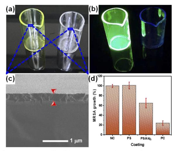
Fig. 9 PS/Alq $_3$  as an antibacterial composite: (a) and (b) 10 ml glass beaker coated with a PS polymer and a PS/Alq $_3$  composite under visible light and UV irradiation ( $\lambda = 385$  nm), respectively; (c) SEM image of the cross-sections of the coated beakers; and (d) histogram demonstrating the MRSA growth ratio after incubation for 24 h in the NC, PS, PS/Alq $_3$  (2% Alq $_3$ ), and PC (5  $\mu$ g ml $^{-1}$ ) group beakers.
