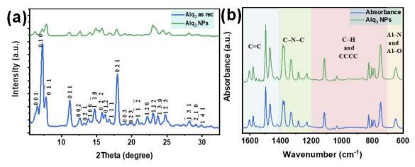
Fig. 4 (a) XRPD patterns and (b) FTIR spectra of the Alq<sub>3</sub> as rec and Alq<sub>3</sub> NP samples' powders.
