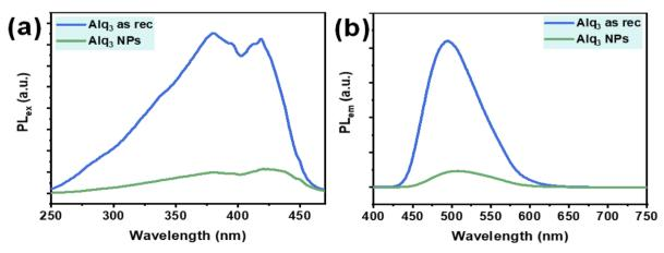
Fig. 5 PL spectra of the Alq<sub>3</sub> as rec and Alq<sub>3</sub> NP samples: (a) excitation spectra ( $\lambda_{em} = 500$  nm) and (b) emission spectra ( $\lambda_{ex} = 380$  nm).
