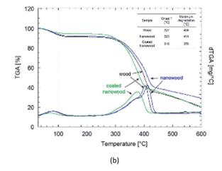
Fig. 3 (a) FTIR-ATR spectra of the wood, nanowood and coated nanowood and (b) shows the thermogravimetrical analysis of the three components with an insert table presenting the onset and max degradation temperatures of each one
