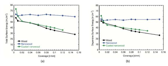
Fig. 4 Comparison of (a) total and (b) dispersive surface energies obtained by IGC from wood, nanowood and coated nanowood samples.
