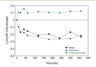
Adsorption kinetic of wood, nanowood and the coated nanowood on a 5.4  $\mu$ g mL<sup>-1</sup> on a solution for 6 h.
