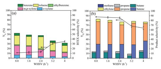
Fig. 8 The liquid (a) and gas yields (b) and selectivity from cracking of LDPE at different WHSV.
