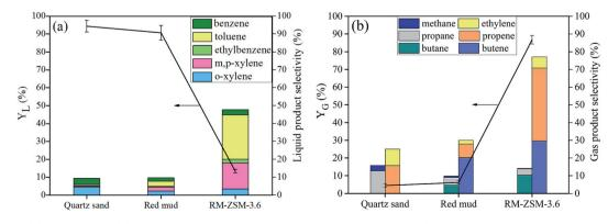
Fig. 9 The liquid (a) and gas yield (b) and selectivity from cracking of LDPE over RM-ZSM-3.6 compared to those over original RM and quartz sand.
